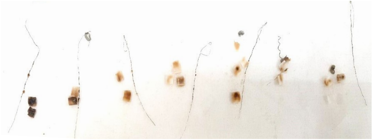
Figure 10: Wicks of resistances obtained during the vaporisation of e-liquids with different PG/VG ratios and each containing 20 mg/mL nicotine and 10 mg/mL sucralose with the Zenith clearomizer. From left to right, the PG/VG ratios are: 100% PG; 80/20; 70/30; 50/50; 30/70; 20/80; 100% VG.
