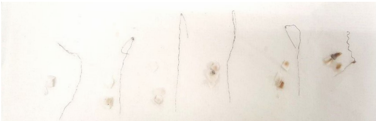
Figure 9: Wicks of resistances obtained during the vaporisation of e-liquids (PG/VG 20/80), nicotine at 20 mg/mL and with different levels of sucralose with the Zenith clearomizer. From left to right, the sucralose concentrations are 1.5, 3, 5, 6.5, 8, 10 mg/mL.
