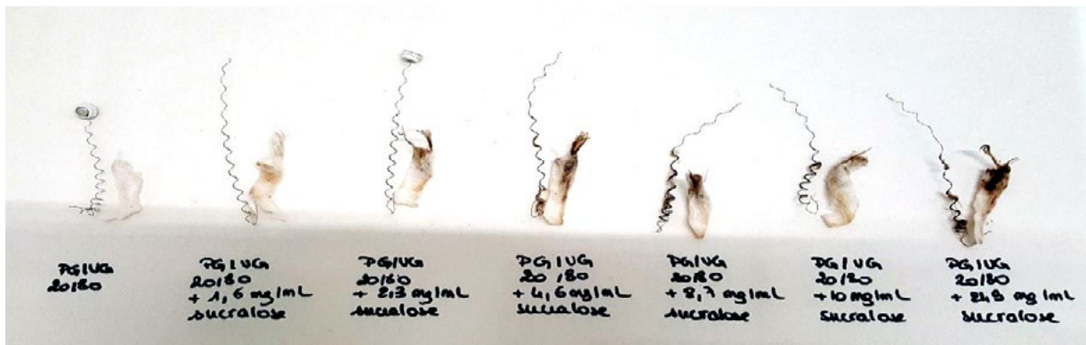
Figure 7: Wicks of resistances obtained during the vaporisation of e-liquids (PG/VG 20/80), nicotine at 20 mg/mL and with different levels of sucralose with the CUBIS clearomizer. From left to right, the sucralose concentrations are 1.6, 2.3, 4.6, 8.7, 10 mg/mL.
